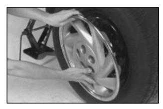
7. If you have a wheel cover, use your fingers to carefully pull the wheel cover from the wheel. Then remove the flat tire.
